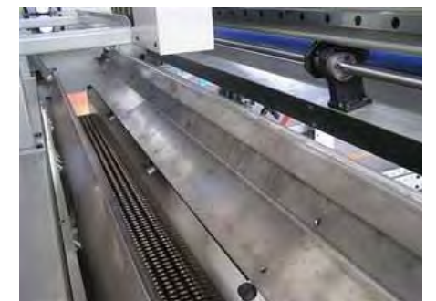
Cut Piece Sorting Sorting system separates usable parts from trim cuts and remnant end.
