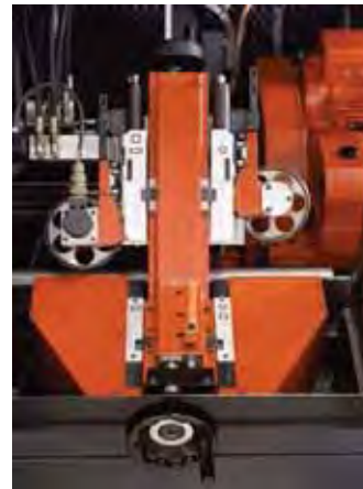
Pinch Roller Feed Easy setting by graduated scale.
