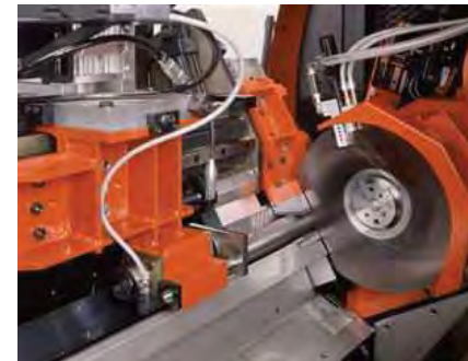
Length Stop Moves at 71"/sec. by servomotor and rack and pinion for just accurate set-up of cut lengths.
