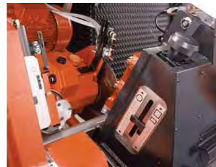
Cutting Head & Vise Powerful 7HP blade driving motor, easy vise adjustment.
