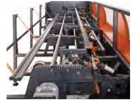
Bundle Storage System Handles all tube, square, and rectangle shape pipes.
